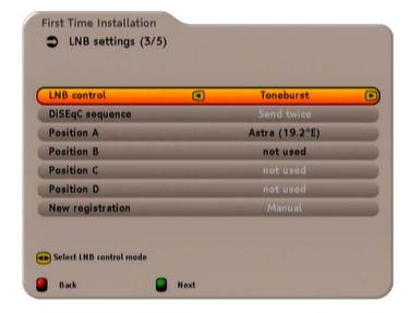
Press the 🔊 buttons to switch to the "Position A". Press the 🕟 button to open the sub-menu. You can select a satellite and make the related settings here. Press the (green) button. If you change the default setting (in this example "ASTRA 19.2°E"), a prompt "Save LNB settings?" will be displayed. Select "Yes" or "No" using the 🕩 buttons and accept your selection using the OK button. Repeat the process as necessary for the second position (B).
